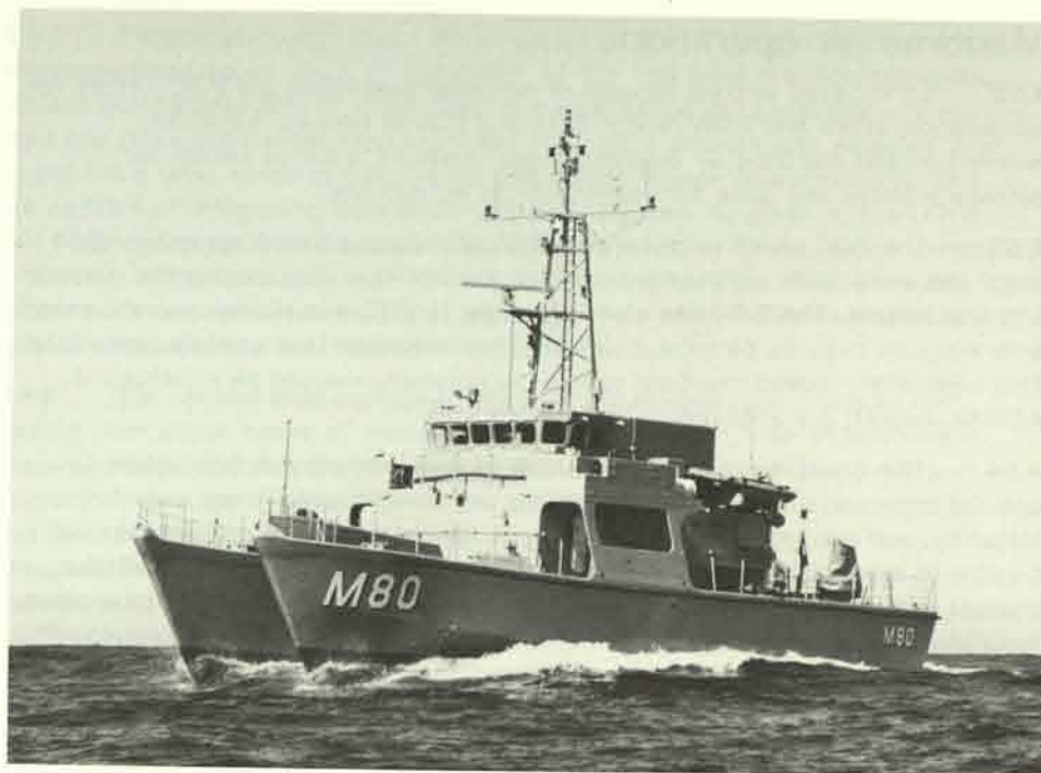
HMAS RUSHCUTTER, a 31 metre glass reinforced plastic catamaran designed to hunt mines in harbours estuaries, channels and other shallow waters which abound along Australia's coastline.
